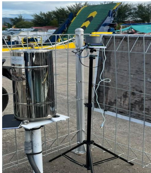
Fig. 3. Hardware Implementation of the Proposed IoT-Based Rainfall Monitoring System
