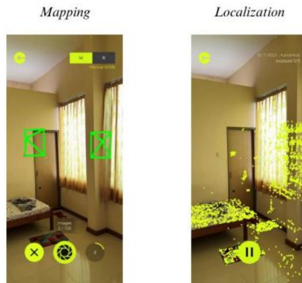
Fig. 2 Mapping and Localization Process Using Immersal Mapper
